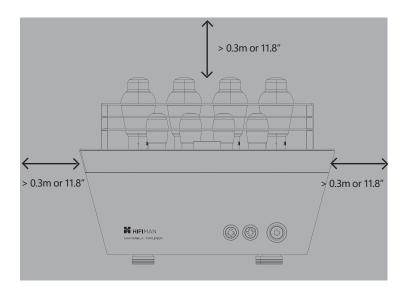
Due to the vacuum tube used inside, the amplifier generates heat. Do not cover the
