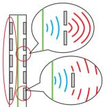
A conventional dynamic driver's frequency response can be altered due to distortions and vibrations across the diaphragm surface.
