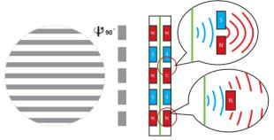
The same happens in conventional electrostatic headphones, where the degradation of sound quality is caused by the stator's interference.
