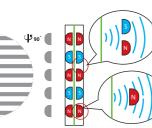
Degradation of sound quality in a conventional planar magnetic headphone is caused by the magnets getting in the way of the sound wave.
