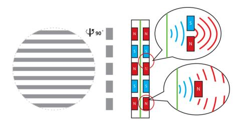
Unlike the sound waves created by a conventional magnet, the special shape of stealth magnet of HE1000 UNVEILED enables the waves to pass through the magnets without generating interference.
